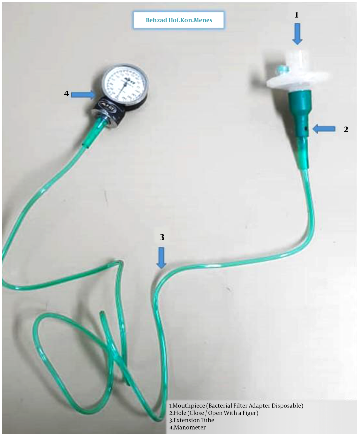
Figure 1. The handmade device used in the present study for the Valsalva maneuver
