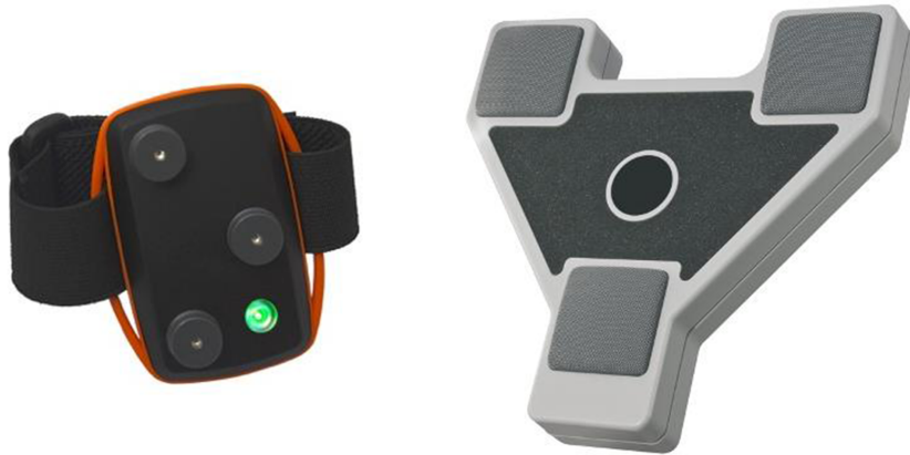
Figure 1. The Wireless Sensor (Left Side; 69 × 23 × 54 mm) and Receiver (Right Side; Size 260 × 250 × 50 mm) of the Ultrasonic System.
