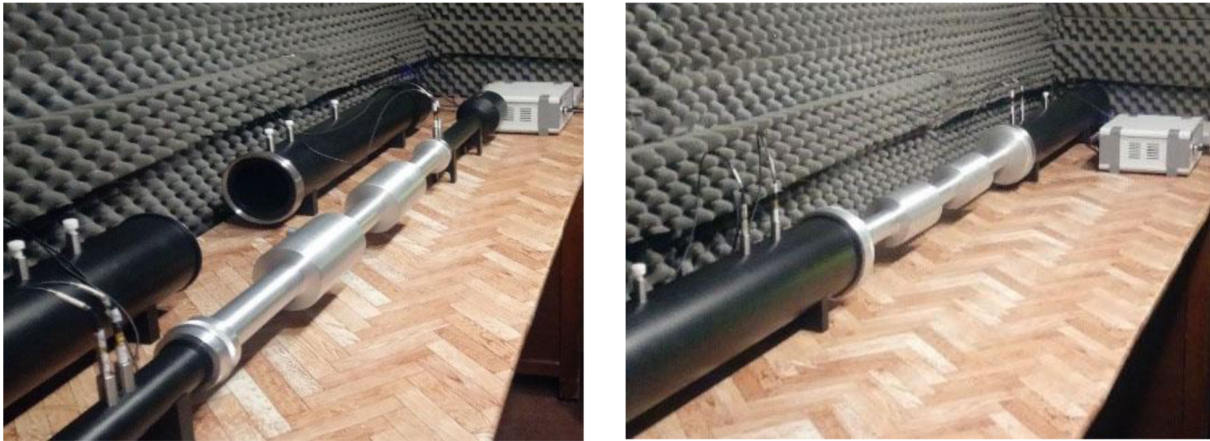
Figure 4. View of the experimental setup for measuring TL; right, low frequencies; left, high frequencies.
