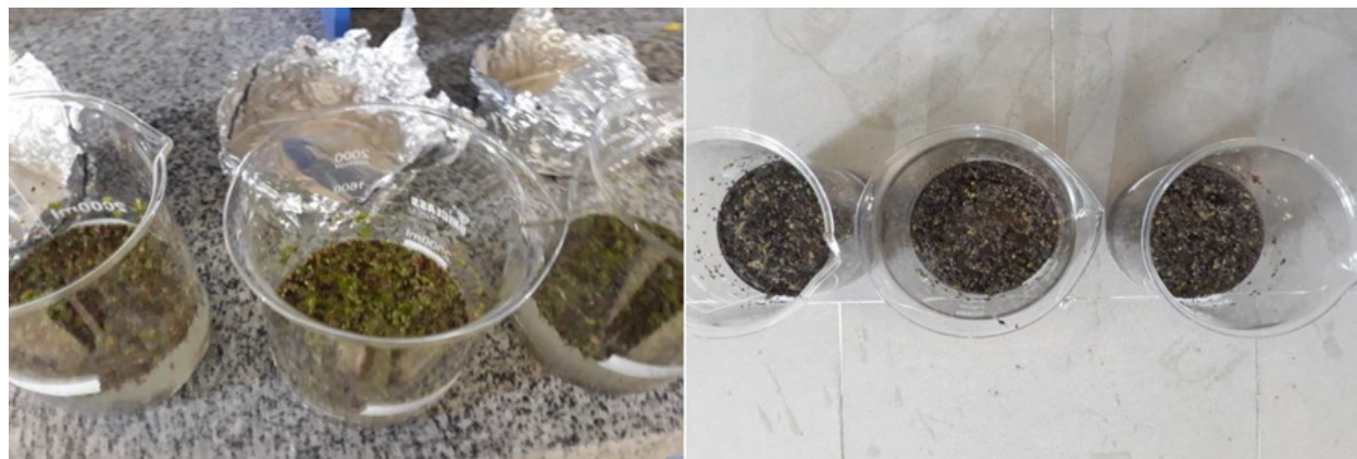
Figure 1. Flasks containing 3.0 grams Azolla and 1000 mgL -1 total petroleum hydrocarbon (TPH): First day (right), after 14 days (left).
