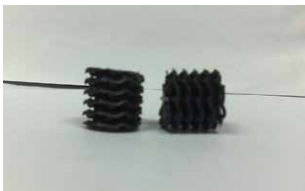
Figure 2. The Media Used in The Experiment With 535 m 2 /m 3 Specific Surface
