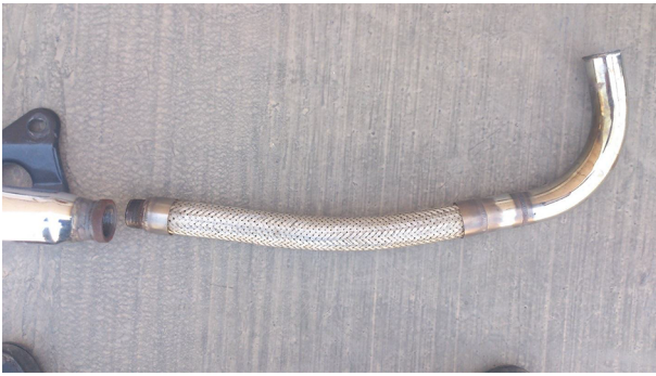
Figure 2. Tailpipe Image Flexible (Flexible Joint)
