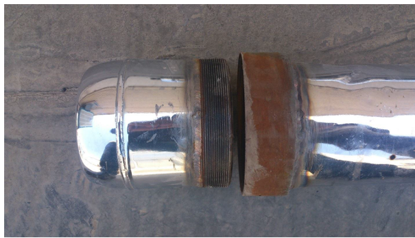
Figure 4. Muffler With the Ability to Open and Close
