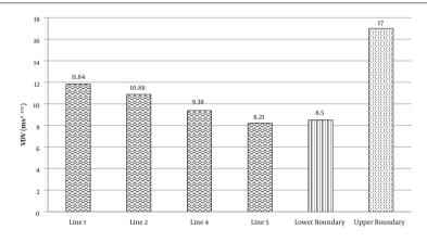
Figure 2. Comparison of means of VDV in different lines lower and upper boundaries of standards
