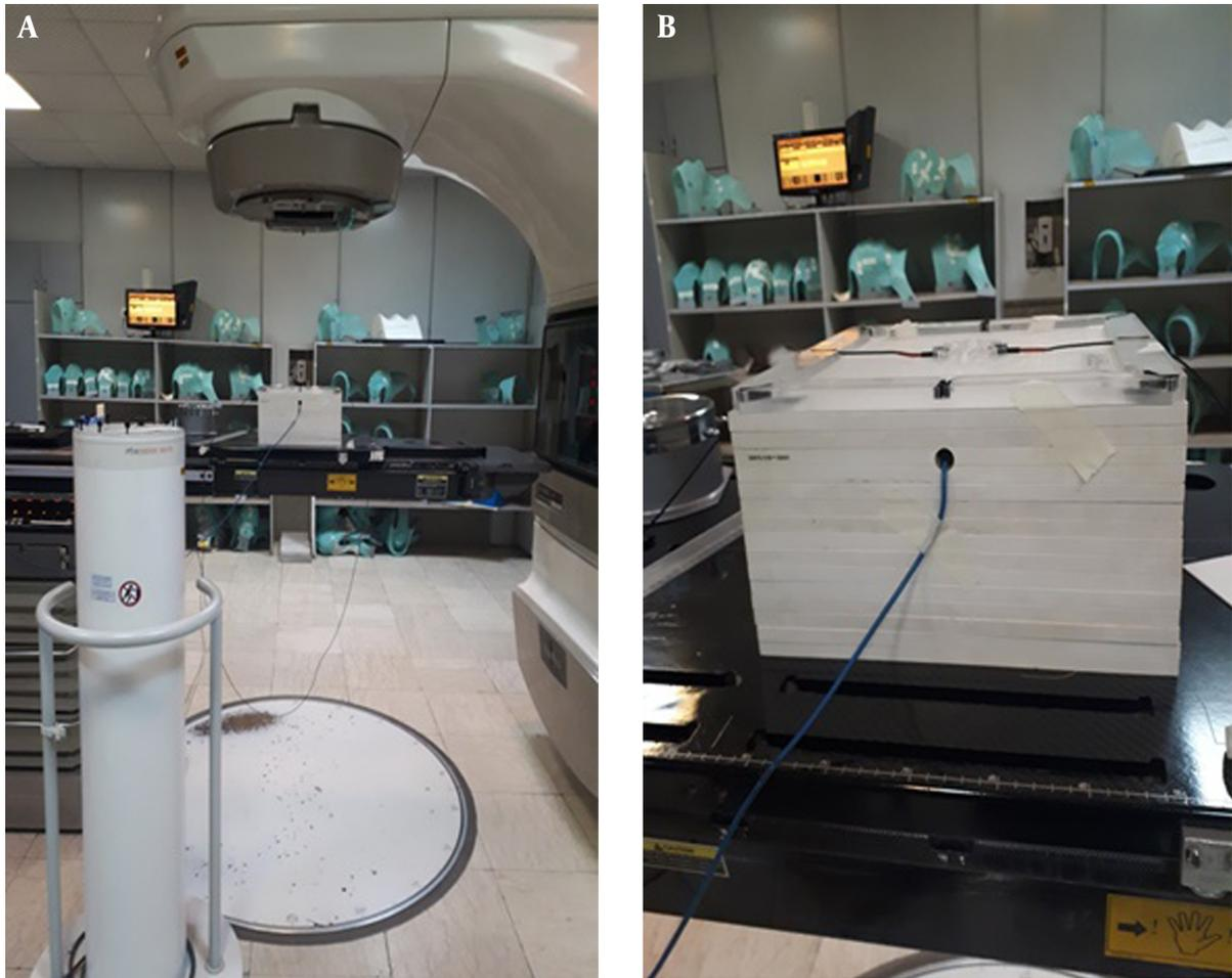
**Figure 1.** A, Illustration of diode system and Linac for in vivo dosimetry; B, Setup for determination of the calibration factor for entrance point by ion chamber
