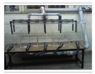
Figure 1. Inhalation Chamber Used for Whole-Body Inhalation Exposure to Carbon Black PM10
