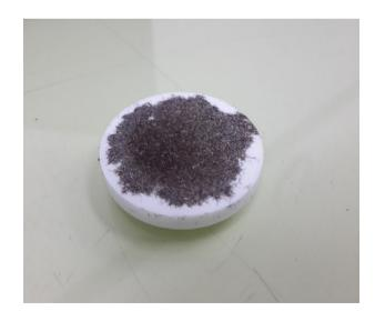
Figure 1. Hair Sample Mounted on Boric Acid
