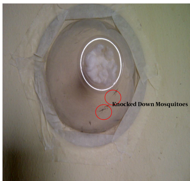
Figure 1. Polyvinyl chloride cone bioassay on the wall painted with the insecticidal paint
