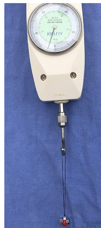
Figure 3. The 3-dimensional-printed attractor can be tightly attached to the bead with the superglue, and the dynamometer reads 25 N before the handle portion is broken.
