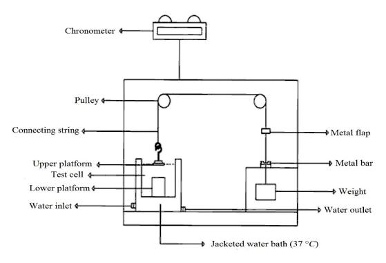
Figure 2. Schematic drawing of one compartment of the apparatus used for assessing the duration of mucoadhesion.
