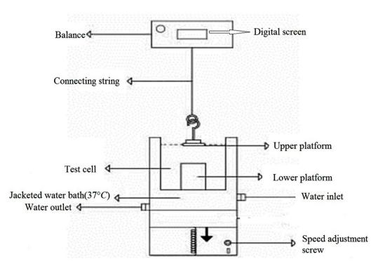
Figure 1. A schematic drawing of the apparatus used for measuring the in-vitro mucoadhesive strength of propranolol HCl formulations.
