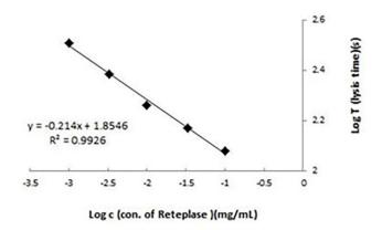
Figure 1. Calibration curve for activated partial thromboplastin time (APTT) lysis test. Lysis times (seconds) were plotted against different concentrations (0.001-0.1 mg/mL) of reteplase standard. Results were the averages of three replicates. Determination of biological activity of recombinant reteplase using clot lysis time and activated partial thromboplastin time (APTT) lysis methods: a comparative study.
