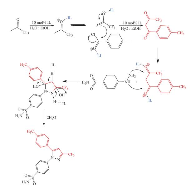
Scheme 3. The suggested mechanism for the synthesis of celecoxib in the presence of ionic liquid.
