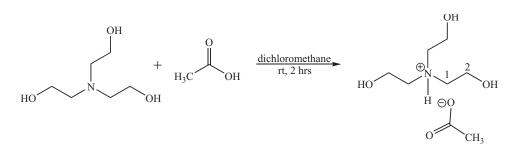
Scheme 1. Synthesis of Tris-(2-hydroxyethyl)ammonium acetate as ionic liquid.
