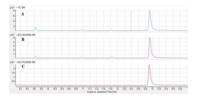
Figure 2. SIM GC-MS total ion chromatogram (A) and extracted ion chromatograms for DBP m/z 149 (B) and DBPd4 m/z 153 (C) in hexane sample (25 ng/ml).
