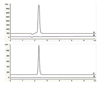
**Figure 3.** Chromatograms of: (A) standard solution, 0.75 mg/mL eptifibatide acetate in 219 nm (B) blank sample (deionized water) in 219 nm (C) standard solution, 0.75 mg/mL eptifibatide acetate in 275 nm (D) blank sample (deionized water) in 275 nm.
