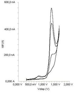
Figure 6. SWV voltammograms obtained for the determination in spiked serum (blank, 5, 10 and 15 µg mL<sup>-1</sup>).
