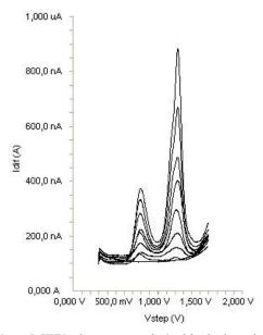
Figure 5. SWV voltammograms obtained for the determination in supporting electrolyte (blank, 1.5, 2.5, 5, 7.5, 10, 12.5, 15 and 17.5  $\mu$ g mL<sup>-1</sup>).
