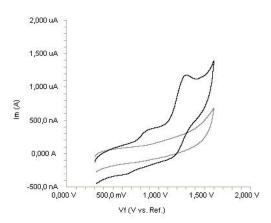
**Figure 2.** Cyclic voltammogram for the oxidation of 20  $\mu$ g mL<sup>-1</sup> diclofenac in acetonitrile containing 0.1 M TBAClO<sub>4</sub> at Pt disk electrode, scan rate: 0.2 V s<sup>-1</sup>.
