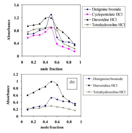
Figure 6. Job's method for distigmine bromide, diaveridine HCl and tetrahydrozoline HCl CT complexes with (a) TCNQ and (b) TCNE reagents in acetonitrile.
