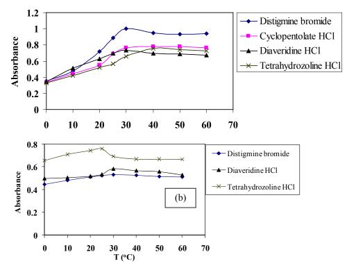
**Figure 5.** Effect of temperature (0-60 °C) on the absorbance of CT complexes of distignine bromide, diaveridine HCl and tetrahydrozoline HCl with (a) TCNQ (t = 30 min,  $\lambda$  = 842 nm) (b) TCNE (t = 30 min,  $\lambda$  = 415 nm) reagents in acetonitrile.
