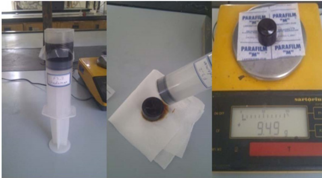
Figure 1. Demonstration of the water absorption content method according to Noda et al.
