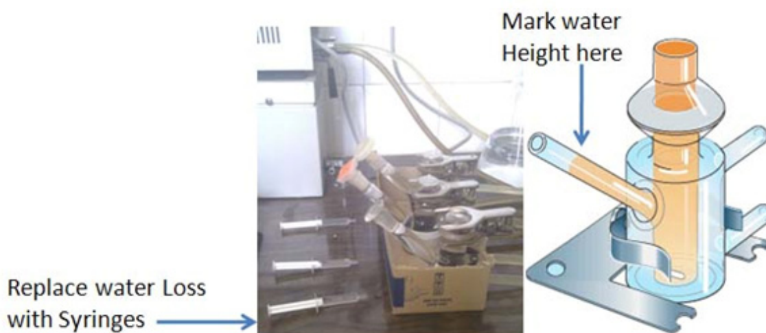
Figure 2. Demonstration of Water absorption rate apparatus according to Noda et al.
