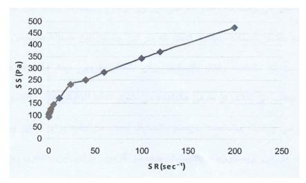
Figure 1. Rheogram of the *a*-tocopherol liposomal gel.SR: Shear Rate; SS: Shear Stress.
