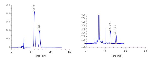
Figure 1. Chromatogram of  $\gamma$ -tochopherol and  $\alpha$ -tochopherol acetate in: a: Calibration standard solution and b: Non branching Naz cultivar sample.
