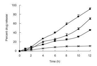
Figure 3. Release profiles of formulations with different amount of CA and PEG 400 Composition of coating membrane: ×, CA: PEG 400 (72.7%:18.2%); ■, CA:PEG 400 (63.6%:27.3%); ▲, CA:PEG 400 (54.5%:36.4%); ●, CA:PEG400 (45.5%:45.5%).
