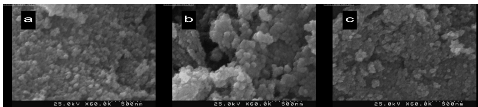
Figure 9. SEM image of MNPs (a), MNPs-COOH (b) and MNPs-COOH-CUR (c).
