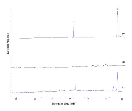
Figure 5. Typical GC–FID chromatograms of: (a) a standard solution prepared in chloroform (100 mg L<sup>-1</sup>, each analyte), (b) drugs free urine, and (c) drugs free urine spiked with the analytes at a concentration of 1 mg L<sup>-1</sup> of each analyte. In chromatogram (a) direct injection was used. In other cases the proposed method was performed on them and 1  $\mu$ L of the final organic phase was injected into the separation system.
