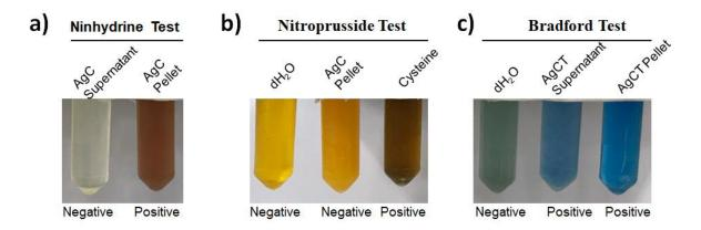
**Figure S1.** Qualitative validation tests for the verification of syntheses (a) Ninhydrin test (b) Nitroprusside test (c) Bradford test.
