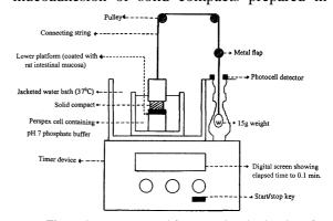
**Figure 1.** Apparatus used for measuring the duration of mucoadhesion of various solid compacts prepared to rat intestinal mucosa (model membrane) at 37°C.
