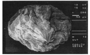
Figure 1. Scanning electron microscopy image of gelatin microspheres.
