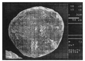
Figure 6. Scanning electron microscopy image of EC-coated microspheres.
