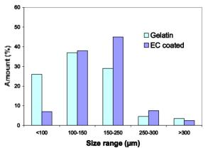
**Figure 3.** Particle size distribution of gelatin microspheres (50:50) and EC (100mg) coated microcapsules
