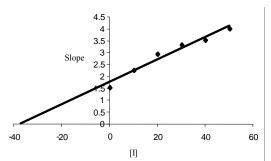
Figure 2-a. Secondary replot of slope from the Lineweaver-Burk plot vs [I]. The X-axis interception at the value of -37 represents the -K  $_{\rm i}$  parameter. [I] values are expressed in  $\mu$ M. R-sq is 0.978.
