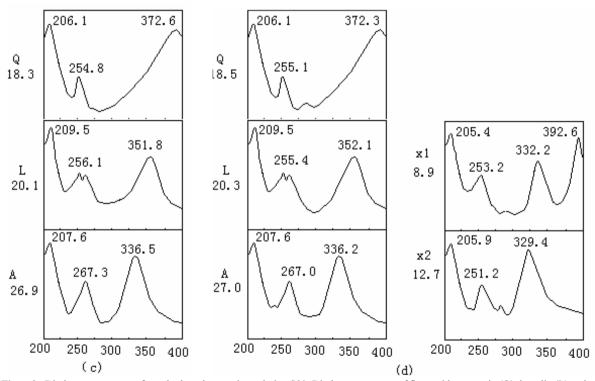
**Figure2.** Diode array spectras of standards and extraction solution S80. Diode array spectra of flavonoids quercetin (Q), luteolin (L) and apigenin (A) were Fig. 2 (a). The UV spectrums of the peaks with retention times of extractive solution S80 were Fig. 2 (b). X1 and x2 were unknown flavonoids.
