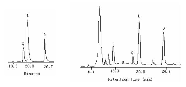
**Figure 1.** HPLC profile at 352 nm. (a) Flavonoids quercetin (Q), luteolin (L) and apigenin (A); (b) extraction solution S80. HPLC system: column, Kromasil RP-C18 column ( $250 \times 4.6$ mm i.d,  $5\mu$ m);mobile phase, methanol-acetonitrile-acetic acid-phosphoric acid-H2O (200:100:10:10:200, *V/V*); detecting wavelength, 352 nm; flow rate, 0.60 ml/min; sensitivity, 0.05 AUFS; quantity volume of injecting sample, 6.0 µl.
