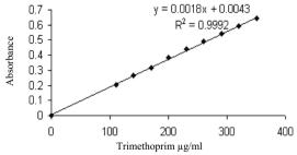
Figure 2. Calibration curve for TMP at 271 nm.
