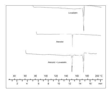
Figure 7. DSC combined thermogram of atenolol and lovastatin.
