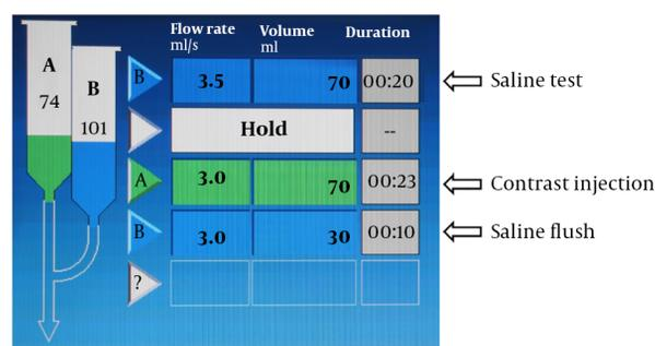
**Figure 1.** Injection protocol on the screen. This is a sample of CT injection protocol for liver tumor detection.
