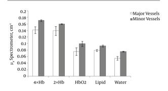
**Figure 3.** Comparisons of absorption coefficients in  $2 \times , 4 \times ,$  and oxy-hemoglobin in the major and minor vessels of the breast phantom using a spectrometer
