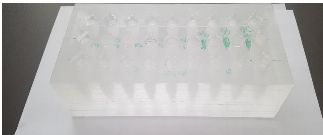
Figure 2. Constructed plexiglas rectangular phantom for imaging gold nanoparticles and iodinated samples
