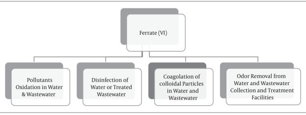
Figure 7. Various Applications of Ferrate(VI) in Water and Wastewater Treatment Technology
