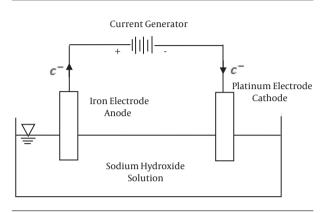
Figure 3. Schematic Representation of the Electrochemical Cell for the Synthesis of Ferrate(VI)
