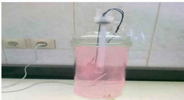
**Figure 1.** Photochemical Reactor
