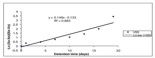
$\label{eq:sigma} \begin{tabular}{ll} Figure 3: Reaction coefficient $k_d$ determination of mixed sludge based on Adams model \\ Jundishapur Journal of Health Sciences, Vol.5, Serial No.2, Summer 2013 \\ \end{tabular}$
