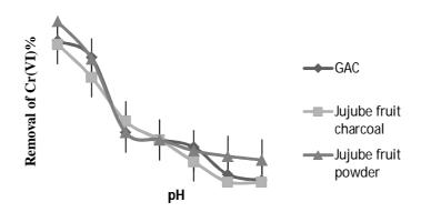
Figure 2: Effect of pH on the removal of Cr (VI) (initial Cr (VI) concentration=1.5 mg/l, adsorbent dose=1.5 g/l contact time= optimum contact time for any adsorbent)
