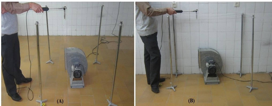
Fig 2: The centrifugal fan as test object located in two locations in the acoustic lab along with the assigned surface
