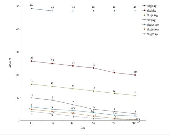
Figure 3. trend of Cr<sup>+6</sup> concentration reduction for all vermicompost pilot of paint sludge and sewage sludge in mg/kg
