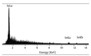
Figure 3. Energy-dispersive X-ray images of purified Se NPs
