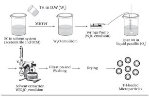
Figure 2. Schematic representation of EC microparticles preparation using double-emulsification the W/O1/O2 method.
