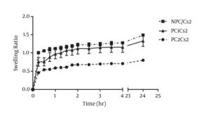
Figure 1. Swelling Ratio of the Films in Phosphate Buffer (pH = 7.4) at 37°C.
