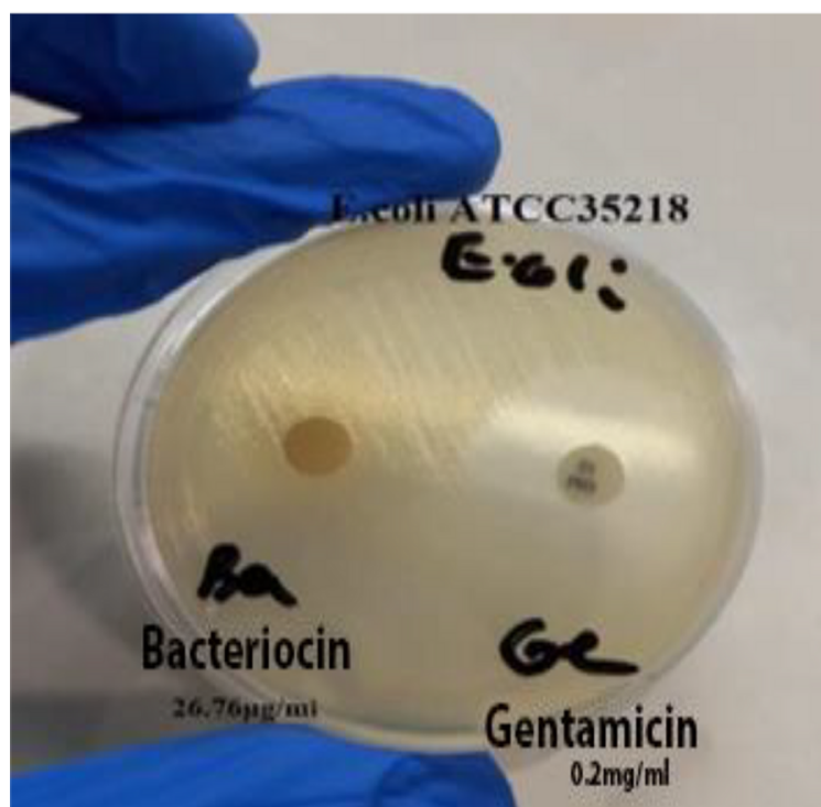
Figure 3. The disc diffusion results of bacteriocin and gentamicin on Escherichia coli ATCC35218
