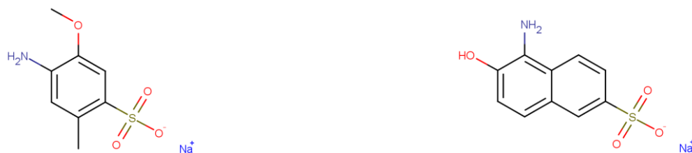
Fig. 7. Chemical structures of two components of AR: 2-methoxy-5-methyl-aniline-4-sulfonic acid (cresidine-4-sulfonic acid) and 1-amino-2-naphthol-6-sulfonic acid.
