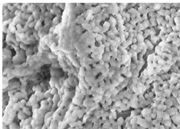
**Fig.4.** SEM images of leaf template Co<sub>3</sub>O<sub>4</sub>.
