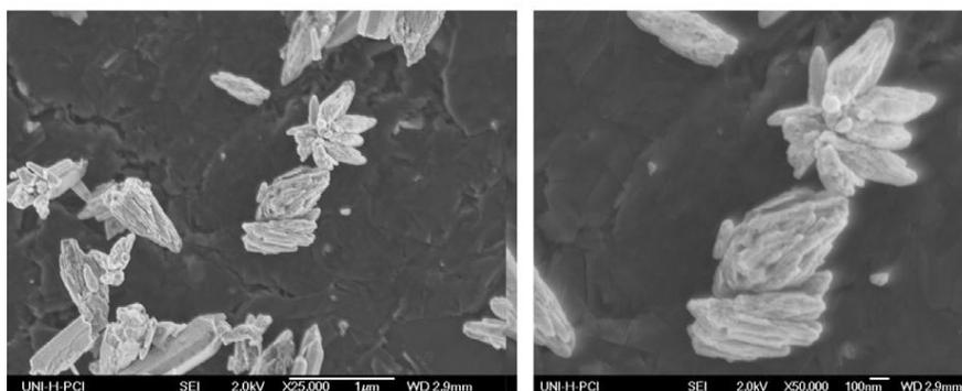
Fig.5. SEM images of flower shape ZnO nanoparticles [77].
