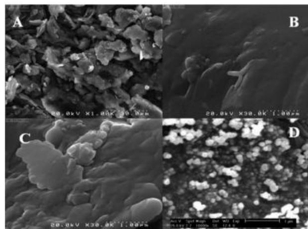
**Fig.1.** SEM images of (1) CPE, (2) CILE, (3) GR-CILE and (4) GR-CILE/Au NPs.
