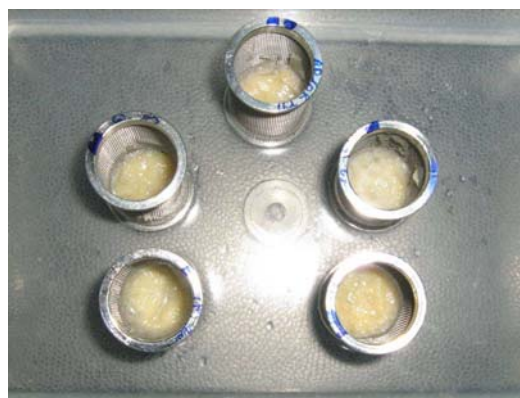
Fig. 1. The designed device for swelling study.
