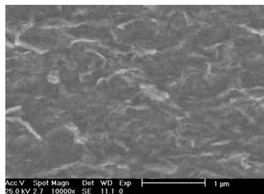
Fig. 2. SEM image of GR-CS/GCE
