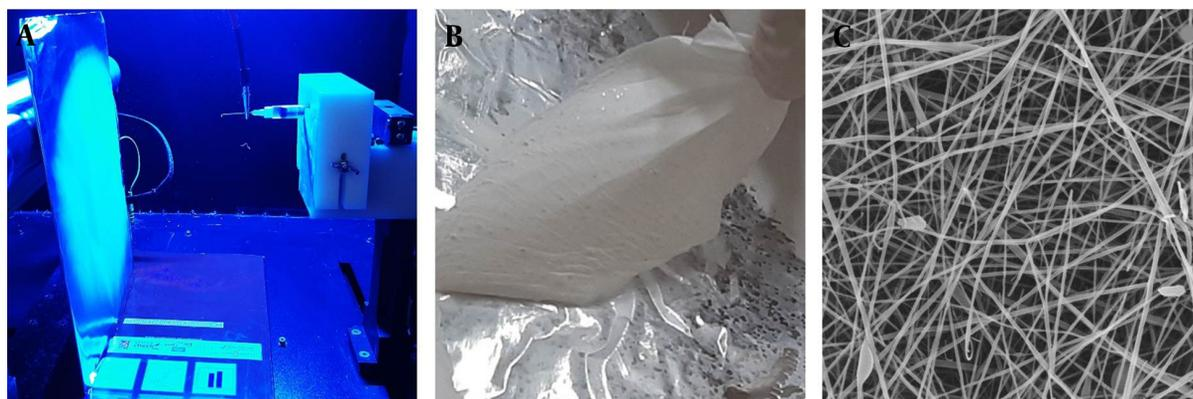
**Figure 2.** A, Fabrication of nanofibrous scaffold by electrospinning method; B, The electrospun silk fibroin nanofiber mat; and C, Field emission scanning electron microscopy image of SF nanofibers
